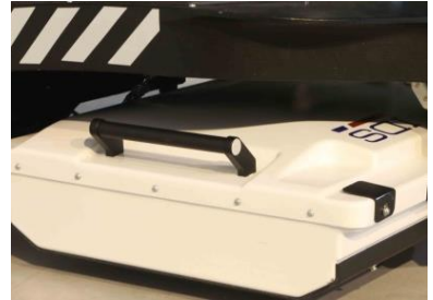
Stream C antenna array
